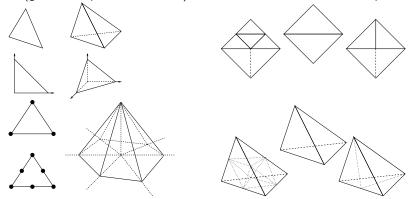
Error-estimate-driven adaptive finite element methods often based on simplex subdivision. (Above: 2/4/8-section and conformity.)
