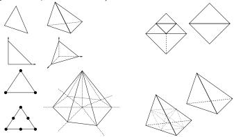
Error-estimate-driven adaptive finite element methods often based on simplex subdivision. (Above: 2/4/8-section and conformity.)
