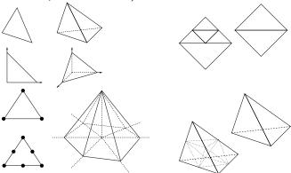
Error-estimate-driven adaptive finite element methods often based on simplex subdivision. (Above: 2/4/8-section and conformity.)
