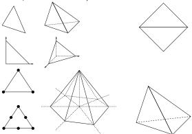
Error-estimate-driven adaptive finite element methods often based on simplex subdivision. (Above: 2/4/8-section and conformity.)
