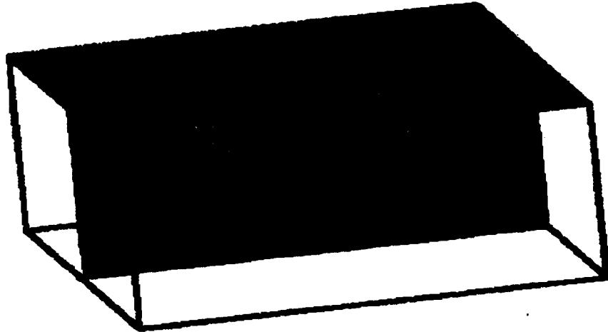
Figure 2: Thermal equilibrium solution. The lighter area is the region of the base which is not depleted in the thermal equilibrium case. The device is 1\ \mu m on a side.
